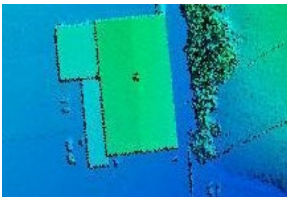
Figure 14. Even with sub-meter NPS, building footprint edges are pixelated. Straight edges are difficult to define when they are irregular and pixelated.
