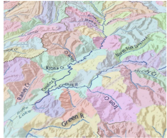
Figure 91. Hydrologic Units and stream networks delineated from an elevation model. Hillshading has been added to show the underlying terrain.
