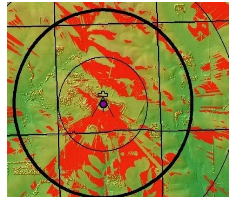
Figure 88. Viewshed map showing what can be seen (red) and not seen (green) from an antenna 9.5 feet tall.
