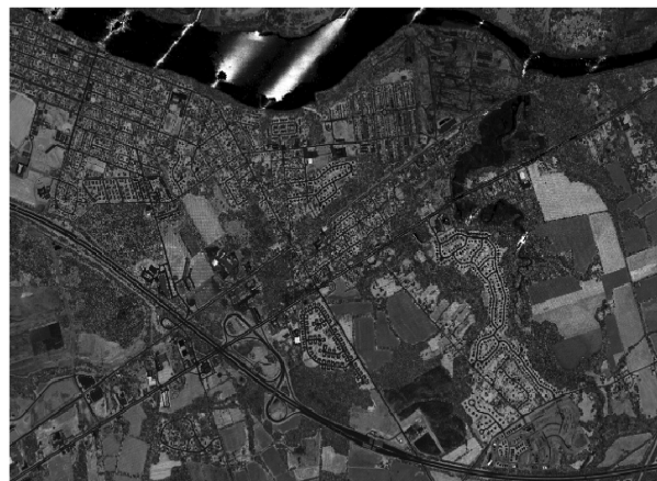
Figure 49. Intensity image showing streaks over water from multiple flight lines. This is not a problem because topographic lidar measurements on water are already assumed to be unreliable and are classified separately as LAS Class 9.
