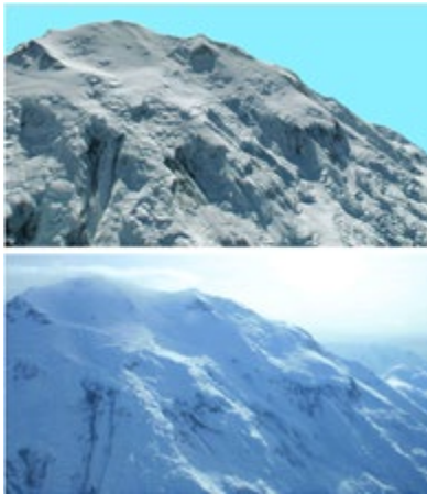
Figure 52. Top: Simulated view of Denali (highest mountain in the U.S.) created by draping a satellite image over the IFSAR DEM. Bottom: Actual fly-by photo of Denali photographed out the window of an aircraft in Alaska.
