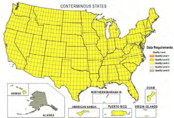
Figure 1.2. Scenario 1, Uniform QL3 LiDAR nationwide except QL5 IFSAR for Alaska; 25-year acquisition period; lowest cost and lowest benefits scenario.
