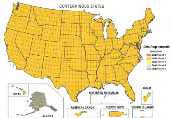
Figure 8.6. Scenario 3, Uniform QL2 LiDAR nationwide except QL5 IFSAR for Alaska; 8-year acquisition period; it has high net benefits and a high B/C Ratio – nearly the same as Scenario 2.
