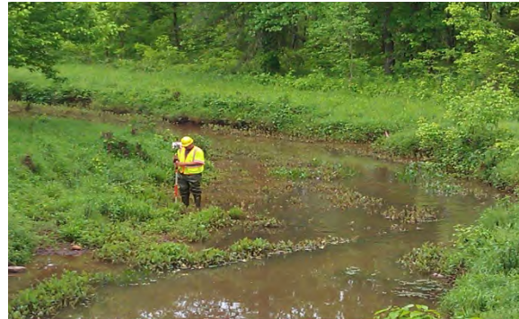
Figure 4.16. Land surveyor surveying stream cross sections in non-navigable waters with conventional survey procedures.
