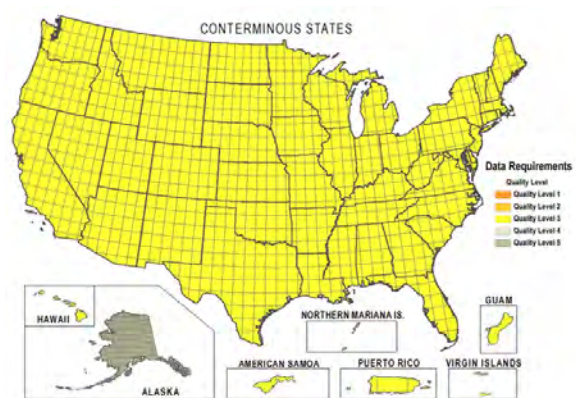
Figure 8.2. Scenario 1, Uniform QL3 LiDAR nationwide except QL5 IFSAR for Alaska; 25-year acquisition period; lowest cost and lowest benefits scenario.
