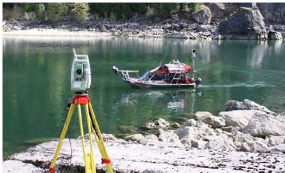
Figure 4.15. Small vessel with sonar that maps bathymetric surfaces in navigable waters that are either clear or turbid.
