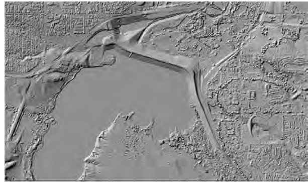
Figure 4.4. Digital Surface Model (DSM) that directly maps the top reflective surfaces of treetops, rooftops, etc.
