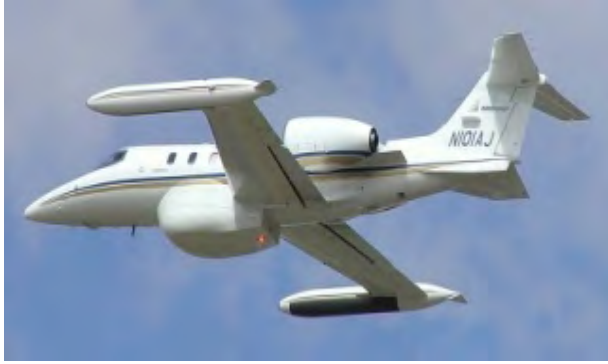
Figure 4.1. IFSAR elevation differences are reconstructed from the phase difference between radar signals arriving at two antennae, with known offsets, housed in the radome.
