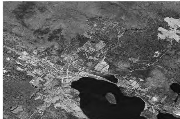
Figure 4.6. A digital orthophoto produced from stereo imagery. Either pushbroom or frame mapping cameras are ideal for digital orthophoto production. Although this is B/W, most orthophotos are full color or color infrared.
