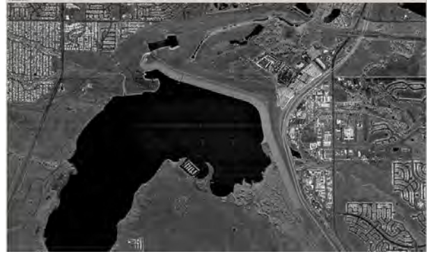
Figure 4.2. Ortho-rectified Radar Image (ORI) is a standard black/white image product of IFSAR. Water returns are black and thus helpful in hydro-enforcement of DTMs.
