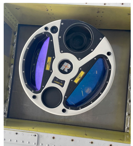
RIEGL VQ-1560 II-S installed on the Cessna T303 Crusader
